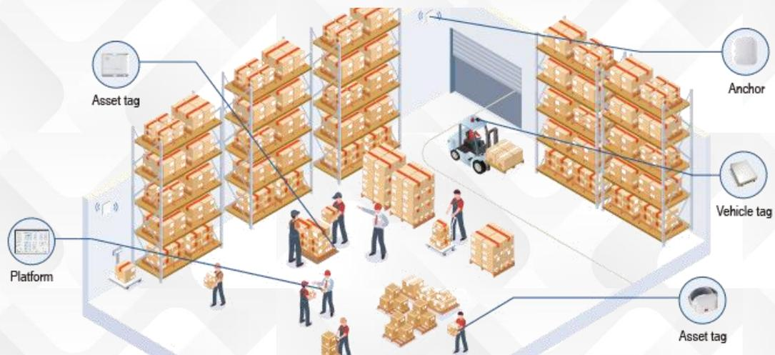
Figure 1: example of RTLS application in a warehouse. Source: <https://www.uwbleader.com/>
